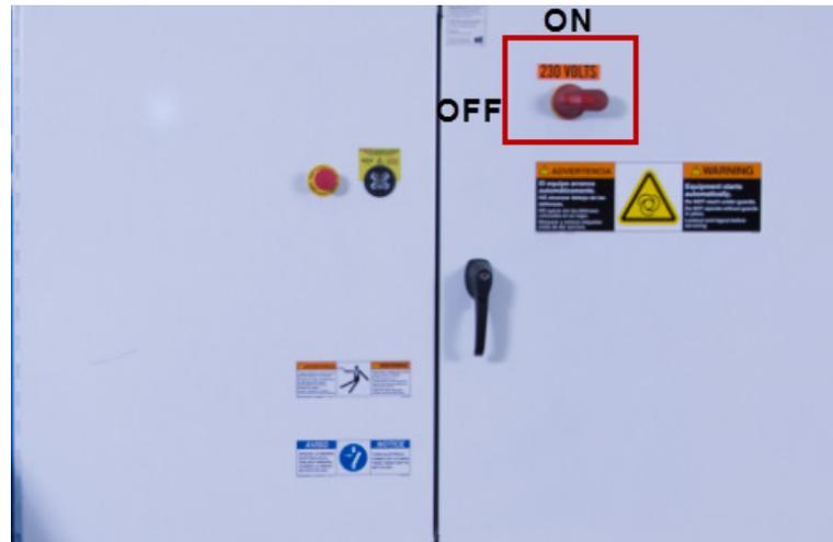
2. Rotate the disconnect switch for the Auto Deck, *WoodRunner*, or other lumber feed or outfeed system (if equipped) to the ON position.
