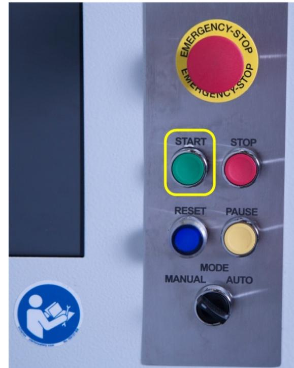
**NOTE:** A common error that occurs when the operator presses **Start Cutting** before starting the saw blade motor. The saw motor must be started before the system will attempt to begin cutting or feeding lumber.
