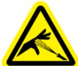
Hydraulic hose is under great pressure. Use safe operating procedures at all times.
