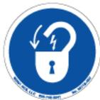
Circuits are live - Lockout/tagout the upstream power source.
