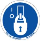
The lock and tag symbol shown to the left indicates that proper lockout/tagout procedures must be used prior to starting the procedure where the symbol occurs.
