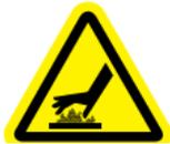
Hot surface! Surface temperature can exceed greater than 70°C during normal operation. Do not touch.
