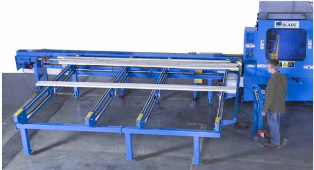
**Figure 2-4: Powered Skewed Conveyor as Part of a *MatchPoint* BLADE System (optional equipment)**
