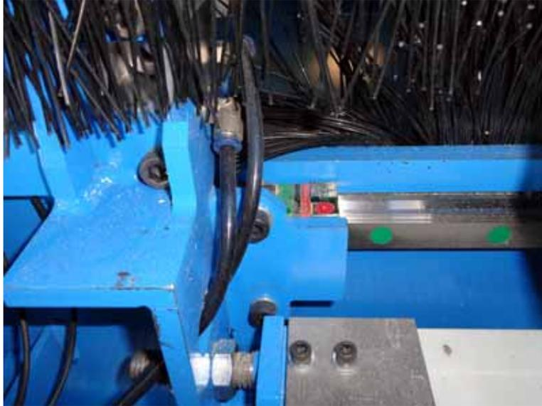
Brushes exist at some openings and rails to keep scrap and other debris from accidentally entering the saw chamber or sitting on a rail causing an axis obstruction. The brushes should be inspected periodically and replaced when necessary.
