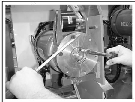
2. To hold the hub in position, fasten two (2) cap screws to the saw hub. They should be the same size as, but not the same ones used on, the saw blade.
