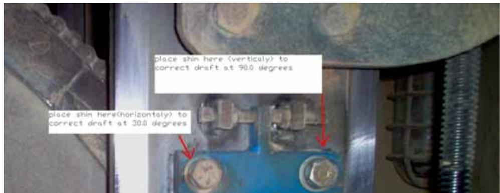
4. Check the pivot point on saw blades 2 and 3.
