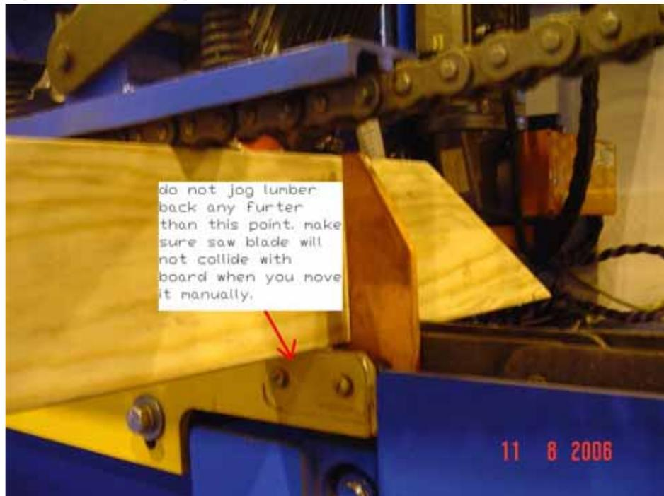
**Figure B-8: Checking Pivot Point**
