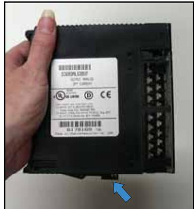
For troubleshooting purposes, you can temporarily switch the suspected bad card with another card of the same type. Use your electrical schematics to determine which slots hold the same type of card.
