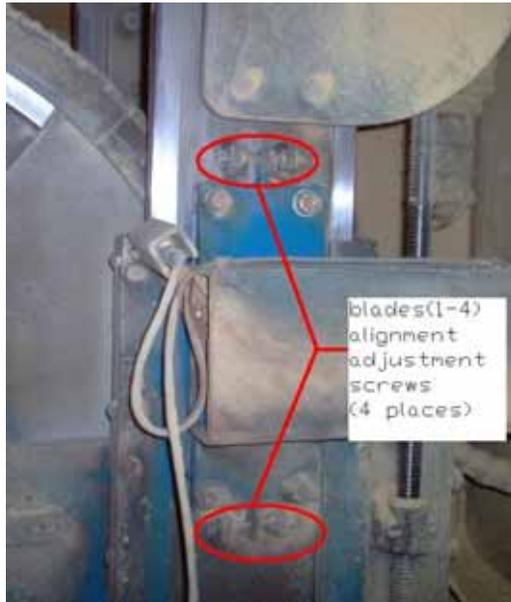
**Figure B-15: Adjusting Blade Alignment Jack Screws**
