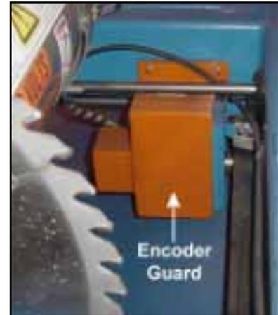
4. Disconnect the defective encoder.
