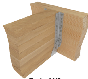
Typical HD installation
