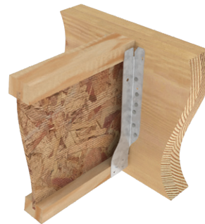
Typical IHFL2514 min nailing installation
